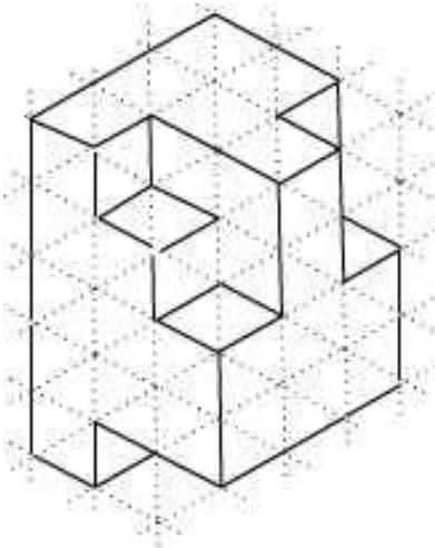
2. Copy this isometric view of a gauge, using the given dimensions. Remember to draw an isometric box! Print the title "Gauge" beneath your drawing.
